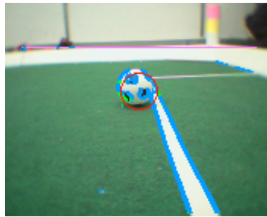
Figure 4.1: Debug-Image. Strong edges are shown in blue. Pixels on the edge of the ball are colored green. The red circle is the result of the Hough transform
